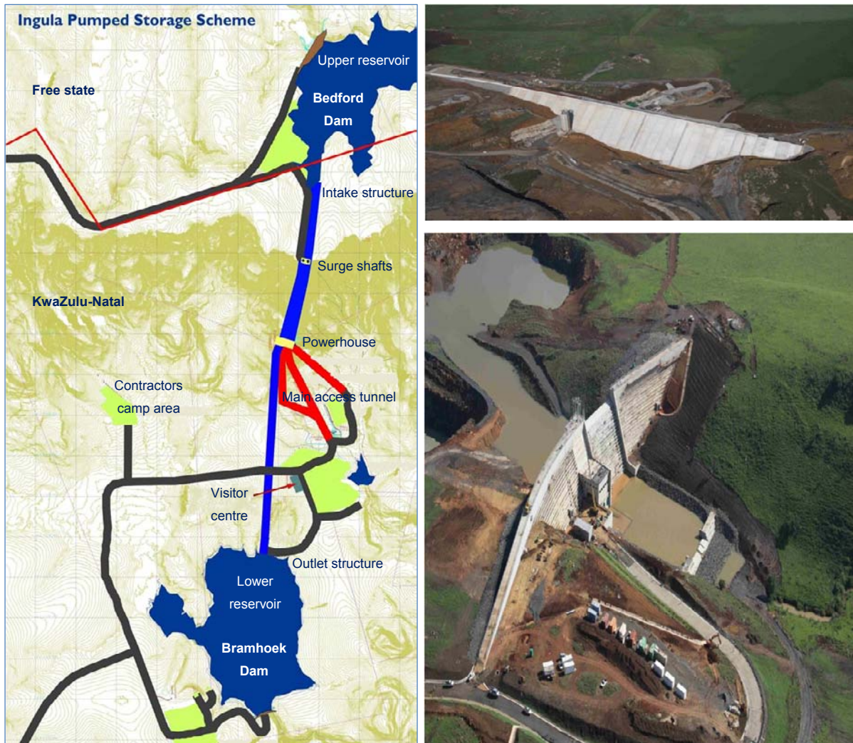
Figure 1. Location Map (left), the upper dam (right top) and the lower dam (right bottom)
