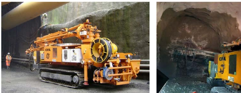
Figure 2. Shotcrete system crawler (left), working in Ingula Site (right)
