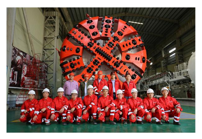
TERRATEC is pleased to announce the delivery of a further two new 6.56m diameter Earth Pressure Balance Tunnel Boring Machines (EPBMs) for the ongoing expansion of Istanbul's Metro system, in Turkey, following successful factory acceptance testing earlier this week. The new EPBMs, along with two other sister machines that have already been delivered to the project, will bring the number of TERRATEC machines working concurrently on the city's metro to a total of nine.
