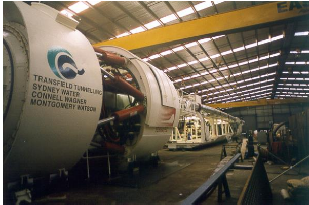
6.0m Double Shield and 3.0m Open TBM delivered in year 2000
