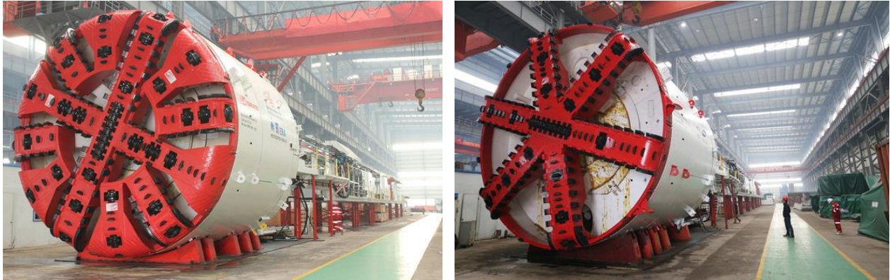
6.61m EPB TBM and 6.52m EPB TBM for Delhi Metro
