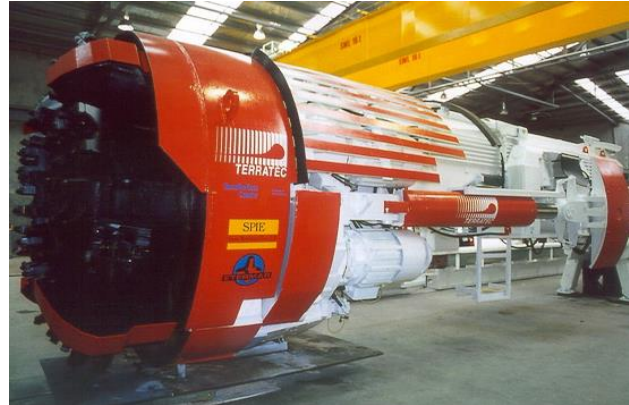
6.0m Double Shield and 3.0m Open TBM delivered in year 2000
