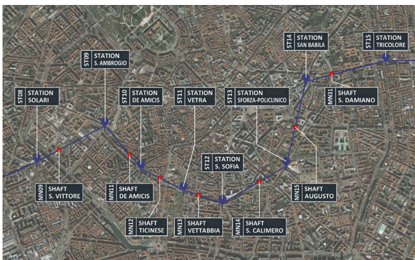
Figure 1. Plan view of the Metro Line 4 City Center stretch.
